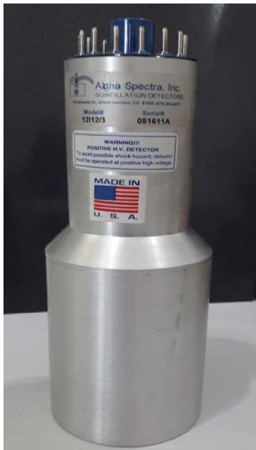
Figure 5: High precision Gamma Detector. Sodium Iodide crystal [NaI(Tl)] doped with Thallium [9].
